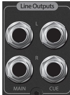
**Main L/R Line Outputs:** Monitor Station V2 passes input audio sources directly to the Main L/R Line Outputs. These outputs derive their signal directly from the currently selected Main input sources and are unaffected by the Main level-control knob and the Mono, Mute, and Dim buttons. Connect these balanced 1/4" TRS jacks to the inputs of a stereo device.
